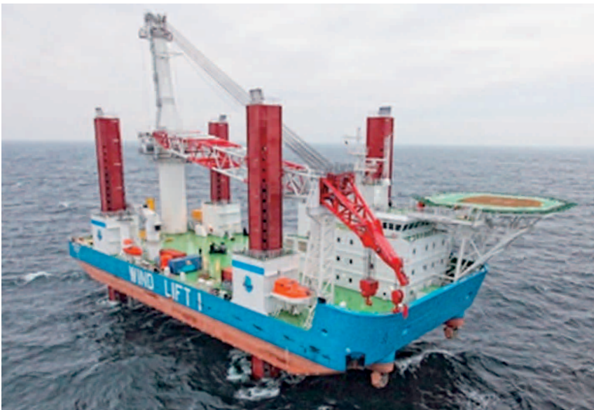
Abb. 3: Jack-Up Plattform © BARD Engineering GmbH
