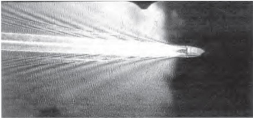
Aerial photograph of wave pattern generated at supercritical speed. The vessel speed is  $V_s = 35$  knots and the water depth is  $h = 13-14$  m. The Froude numbers are  $F_{nh} \sim 1.5$  and  $F_{nl} \sim 0.7$ . The overall length of the catamaran is approximately 78 m.
