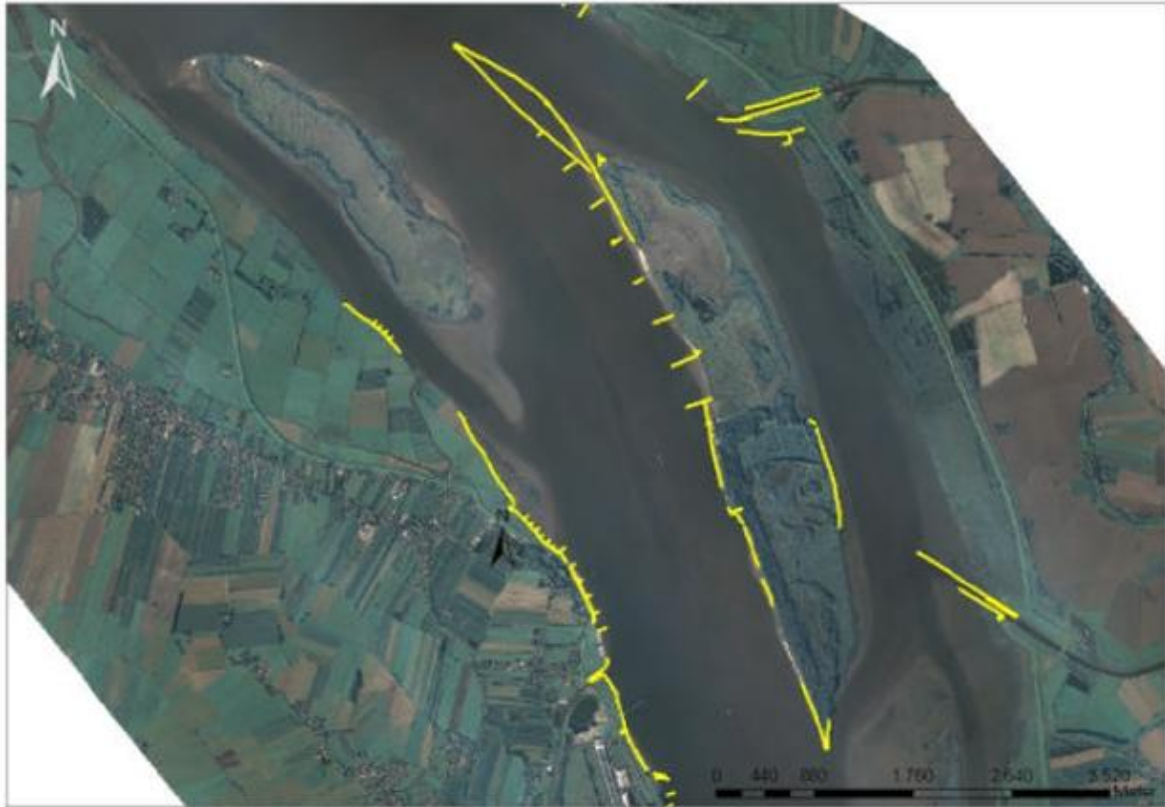
Figure 6: Aerial photograph of Schwarztonnensand (left) and Pagensand (right) showing different concepts of groins and revetments (yellow) protecting tidal marshes from erosion (from Witte & Eichweber (s.d.).
